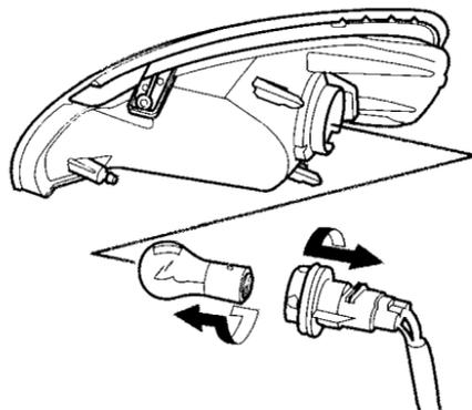
3. Turn the socket one-quarter turn counterclockwise to remove it from the lens.
