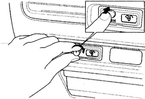
The knob on the dashboard to the left of the steering column controls the brightness of the instrument panel lights. Push the knob to get it to pop out. Turn the knob to adjust the brightness. Push the knob back in to lock your adjustment.
