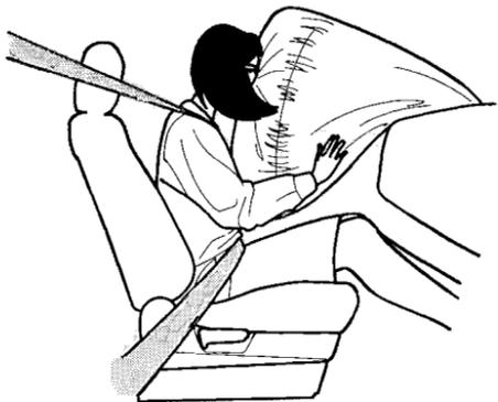
If you ever have a severe frontal collision, the passenger's airbag will inflate at the same time as the driver's airbag.
