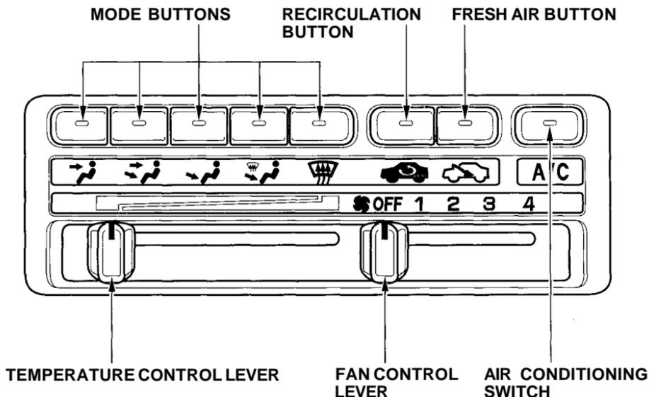
These settings direct all the air flow to the defroster vents at the base of the windshield and the side window defroster vents. The air flow will get warmer and clear the windows faster as the engine warms up. You can close the corner vents with the dial beside each vent. This will send more warm air to the windshield defroster vents.
