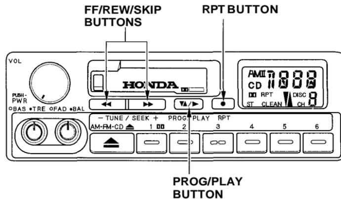
**REPEAT** — The Repeat function continuously replays the current song or passage. Press the RPT button to activate it; you will see RPT displayed as a reminder. When the system reaches the end of the song or passage currently playing, it will automatically go into rewind. When it senses the beginning of the same song or passage, the system returns to PLAY mode. It will continue to repeat this same program until you deactivate REPEAT by pressing the button again.
