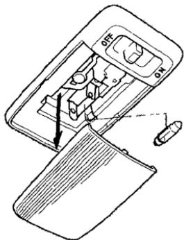
2. Remove the bulb by pulling it straight out of its metal tabs.
