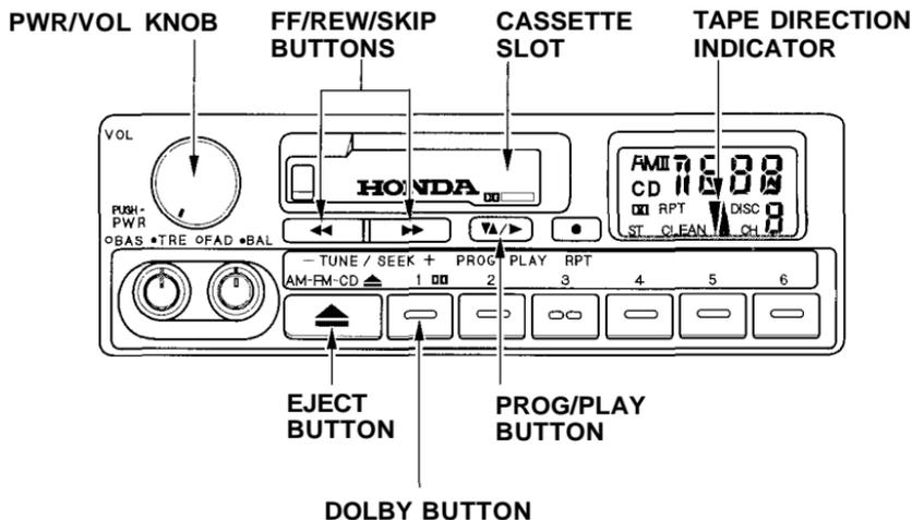
When the system reaches the end of the tape, it will automatically reverse direction and play the other side. If you want to remove the cassette from the drive, press the EJECT button.
