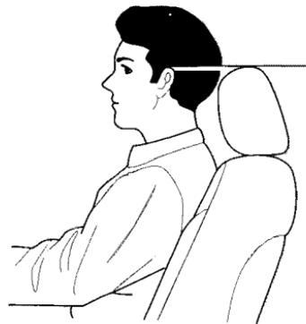
Head restraints can help protect you from whiplash and other injuries. For the best protection, adjust the top of the restraint so it is even with the tops of your ears, or as high as possible. For instructions on adjusting the head restraints, see page [56](#).
