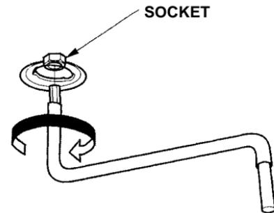
5. Insert the sunroof wrench into the socket behind this plug. Turn the wrench until the sunroof is fully closed.
