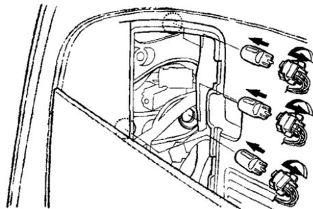
3. Remove the socket by turning it one-quarter turn counterclockwise.
