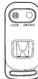
You can lock and unlock your vehicle with the remote transmitter. When you push the LOCK button, all doors and the tailgate lock.
