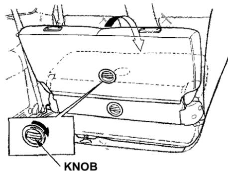
2. Unlock the seat-back by turning the knob. Push the seat-back forward.
