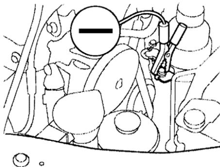
4. Connect the second jumper cable to the negative ( — ) terminal on the booster battery. Connect the other end to the grounding strap as shown. Do not connect this jumper cable to any other part of the engine.
