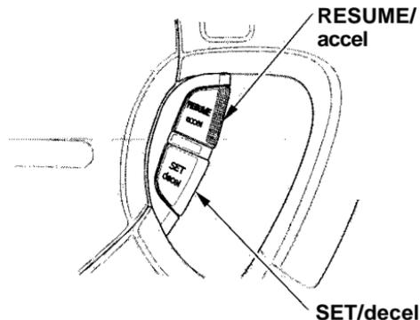
3. Press and hold the SET/decel button on the steering wheel until the CRUISE CONTROL light on the instrument panel comes on. This shows the system is now activated.
