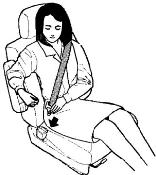
1. Pull the latch plate across your body and insert it into the buckle. Tug on the belt to make sure the latch is securely locked.
