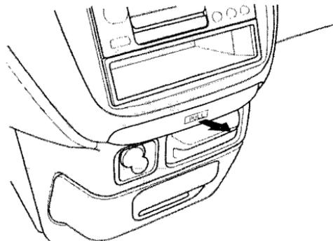
To use the front beverage holder, pull on the front. Push the holder all the way in to close it.
