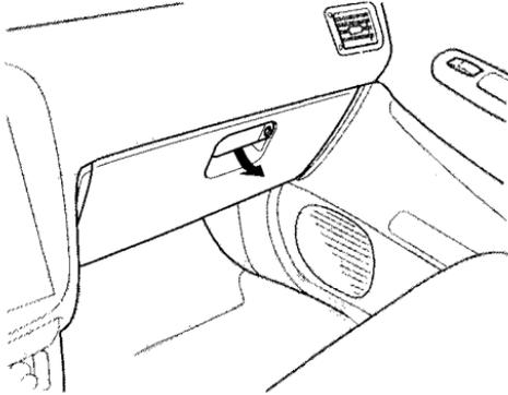
Open the glove box by pulling the bottom of the handle. Close it with a firm push. Lock or unlock the glove box with the master key.
