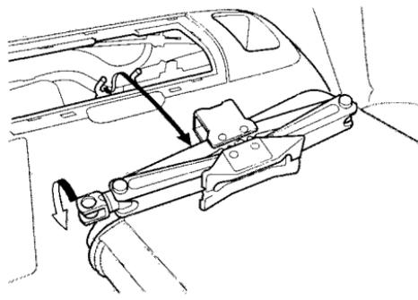
5. Remove the tools from the tray. Remove the tray by pulling it straight up.
