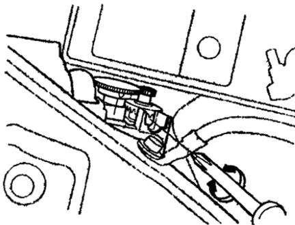
6. If either indicator is not aligned with its "0" mark as described, an adjustment can be made using a Phillips-head screwdriver to realign it with the "0" mark. Please refer to the illustrations.
