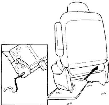
Unhook the front of the seat from the floor by pulling it back slightly, then pivoting it upward.
