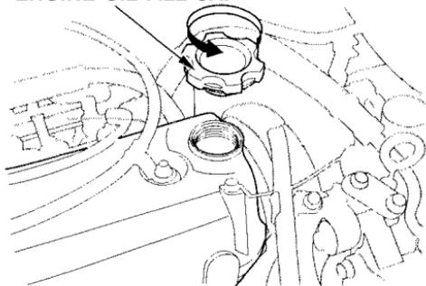
To add oil, unscrew and remove the engine oil fill cap on top of the valve cover. Pour in the oil, and replace the engine oil fill cap. Tighten it securely. Wait a few minutes and recheck the oil level. Do not fill above the upper mark; you could damage the engine.
