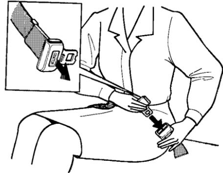
1. Pull the latch plate across your hips and insert it into the buckle marked CENTER.
