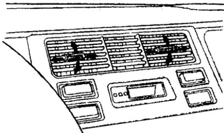
You can adjust the direction of the air coming from the dashboard vents by moving the tab in the center of each vent up-and-down and side-to-side.
