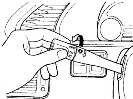
The rotating switch on the left lever controls the lights. Turning this switch to the "OFF" position turns on the parking lights, taillights, instrument panel lights, side-marker lights, and rear license plate lights. Turning the switch to the "HEADLIGHTS" position turns on the headlights.
