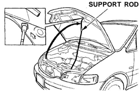
3. Pull the support rod out of its clip and insert the end into the hole on the left side of the hood.
