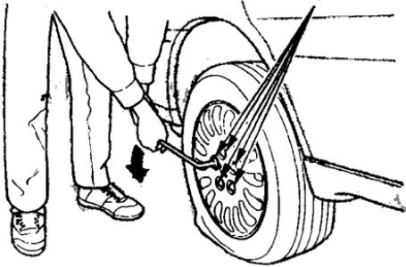
9. Loosen the five wheel nuts 1/2 turn with the wheel wrench.
