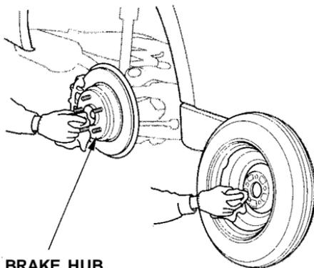
13. Before mounting the spare tire, wipe any dirt off the mounting surface of the wheel and hub with a clean cloth.
