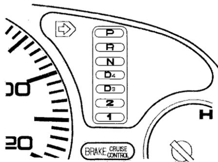
This indicator on the instrument panel shows which shift position the shift lever is in.
