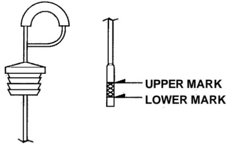
3. Insert the dipstick all the way into the transmission.
