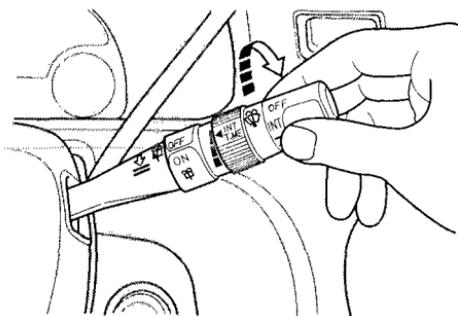
The right lever controls the windshield wipers and washers. The rotary switch at the end of the lever has three positions:
