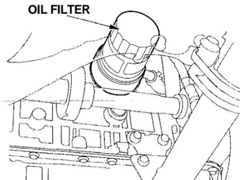
3. Remove the oil filter and let the remaining oil drain. A special wrench (available from your Honda dealer) is required to remove the filter.
