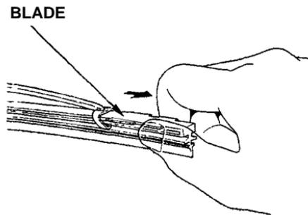
3. Remove the blade from its holder by grasping the tabbed end of the blade. Pull firmly until the tabs come out of the holder.
