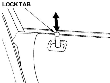
Each door also has a lock tab on the top. When you push down the lock tab on the driver's door, all the doors and the tailgate lock. Pulling up the lock tab on the driver's door unlocks only that door. The lock tab on each passenger's door locks and unlocks only that door.
