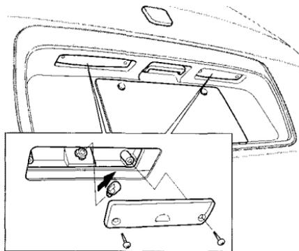
1. Remove the two screws and remove the lens.
