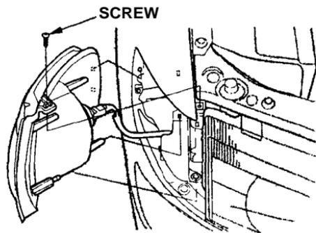
1. Use a Phillips-head screwdriver to remove the screw from the top of the fender.
