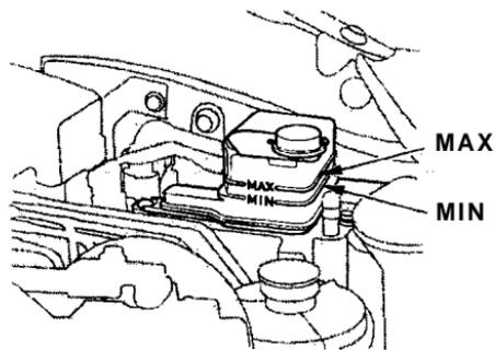
The fluid should be between the MIN and MAX marks on the side of the reservoir. If it is at or below the MIN mark, it indicates a possible problem in the ABS. Have the dealer inspect the system as soon as possible.
