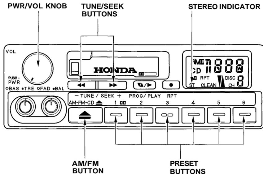
You can use any of three methods to find radio stations on the selected band: TUNE, SEEK, or the Preset buttons.
