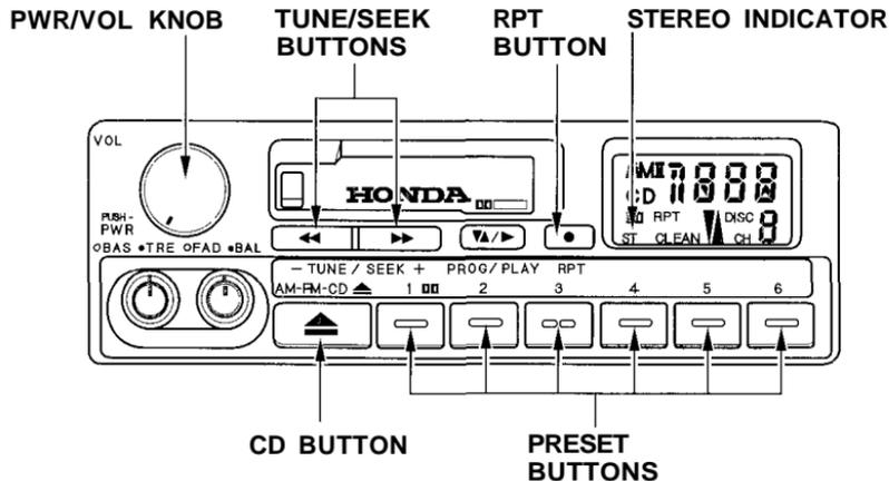
To operate the CD changer, the ignition must be in ACCESSORY (I) or ON (II) and the audio system must be on. If you are listening to a cassette, eject it.
