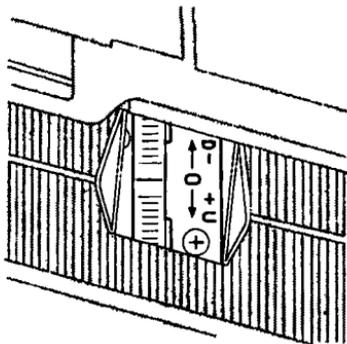
5. Check the vertical angle gauge. The bubble should be centered underneath the longest scribe mark on the gauge.
