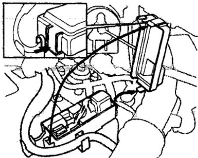
The ABS fuse box is in the engine compartment on the right side.
