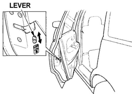
The childproof door locks are designed to prevent children seated in the rear from accidentally opening the rear doors. Each rear door has a lock lever near the edge. With the lever in the LOCK position, the door cannot be opened from the inside regardless of the position of the lock tab. To open the door, pull the lock tab up and use the outside door handle.
