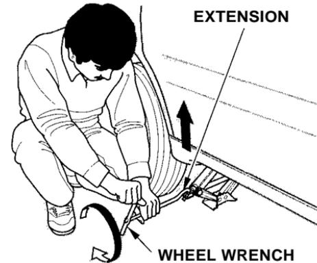
11. Use the extension and wheel wrench as shown to raise the car until the flat tire is off the ground.
