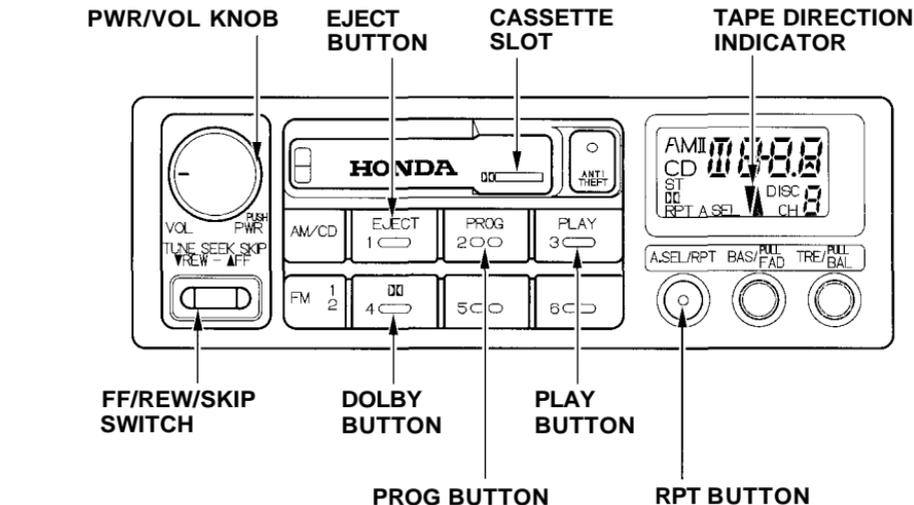
When the system reaches the end of the tape, it will automatically reverse direction and play the other side. If you want to remove the cassette from the drive, press the EJECT button.
