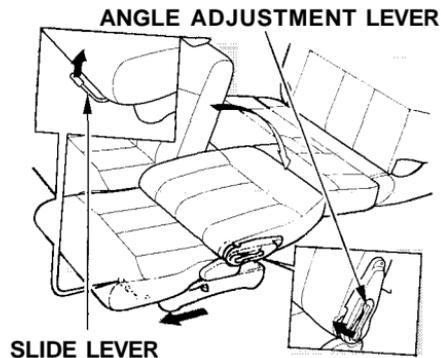
2. Lift the lever and slide the seat forward as far as it will go. Pull the seat-back angle adjustment lever and pivot the seat-back backward. Release the lever when the seat-back is even with the cushion on the third seat.
