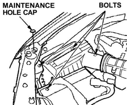
3. Loosen the four bolts and remove the air cleaner housing cover. Remove the maintenance hole cap so you can reach the right front bolt through the hole.
