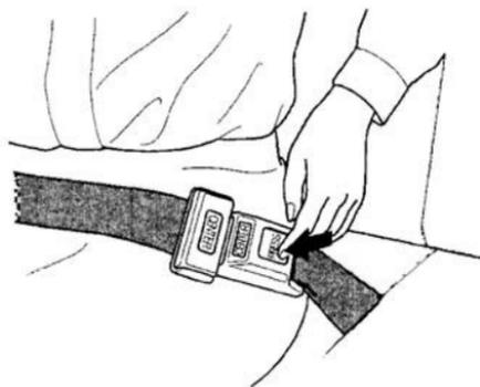
To unlatch the belt, push the red PRESS button on the buckle.
