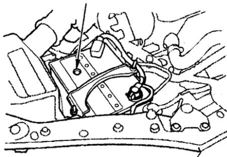
Check the battery condition by looking at the test indicator window on the battery. The label on the battery explains the test indicator's colors.
