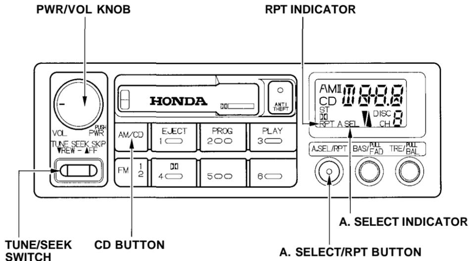
Press the CD button until "CD" appears in the display. The system will start to play the first track of the first disc in the magazine. When that disc ends, the next disc in the magazine is loaded and played. After the last disc finishes, the system returns to disc 1.
