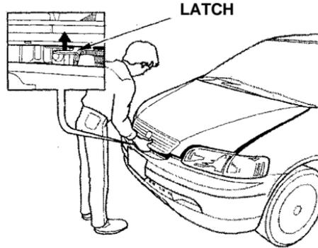
2. Standing in front of the car, put your fingers under the front edge of the hood to the right of center. Slide your hand to the left until you feel the hood latch handle. Push this handle up until it releases the hood. Lift the hood.
