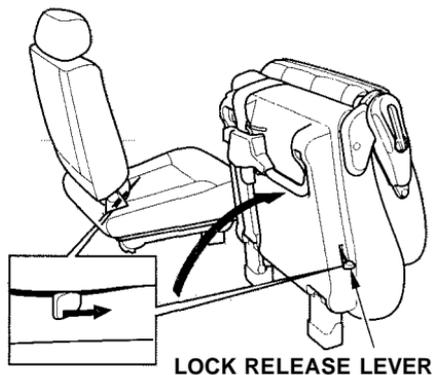
Pull the seat-back angle adjustment lever on the second row seat to tilt the seat-back forward. Pull the lock release lever and pivot the seat up out of the way.
