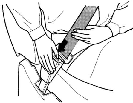
To unlatch the seat belt, push the red PRESS button on the buckle. Guide the belt across your body to the door pillar.
