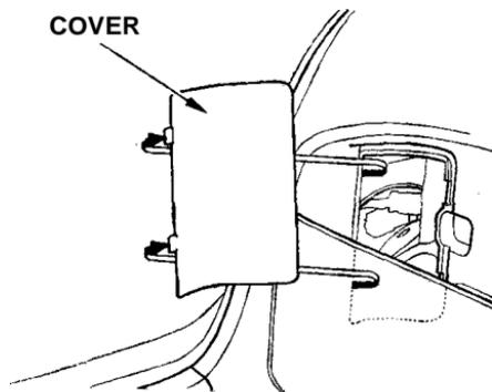
1. Open the tailgate. Swing the taillight cover open and remove it. To replace a bulb on the right side, remove the spare tire (see page [196](#)).
