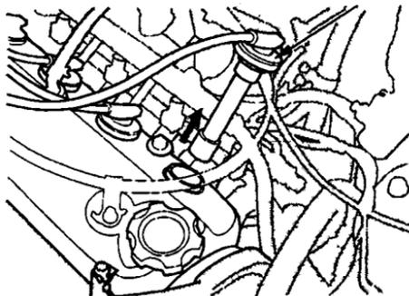
1. Clean up any dirt and oil around the spark plug caps.
