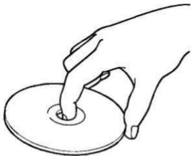
Handle a CD by its edges; never touch either surface. Contamination from fingerprints, liquids, felt-tip pens, and labels can cause the CD to not play properly, or possibly jam in the drive.
