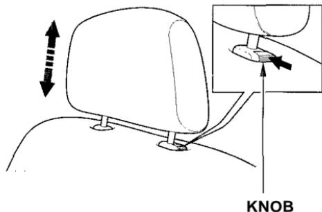
The head restraints are designed to help reduce the risk of neck injuries. Your Honda has adjustable head restraints in all the outside seating positions. Adjust the head restraint so the top is even with the tops of your ears.
