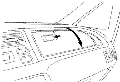
Open the dashboard compartment by squeezing the handle. Close it with a firm push.
