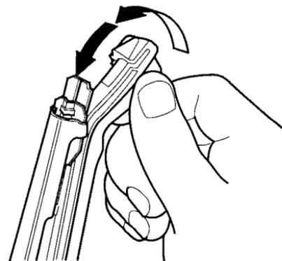
6. Insert both ends of the blade into the holder slots. Make sure they are secure.
