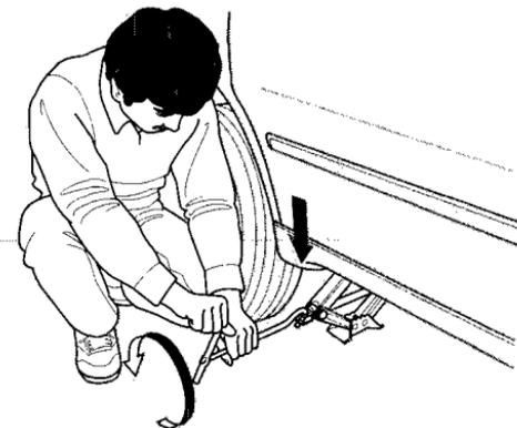
15. Lower the car to the ground and remove the jack.
