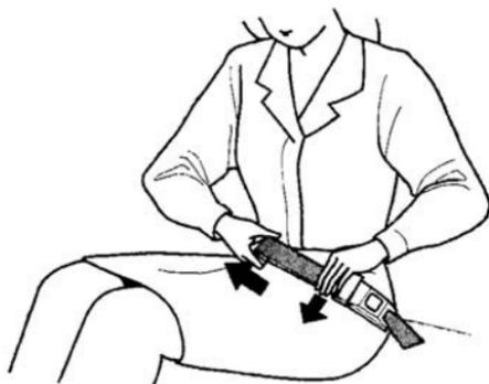
2. Position the belt as low as possible across your hips and pelvic bones, not across your stomach. Pull the loose end of the belt to adjust for a snug but comfortable fit.
