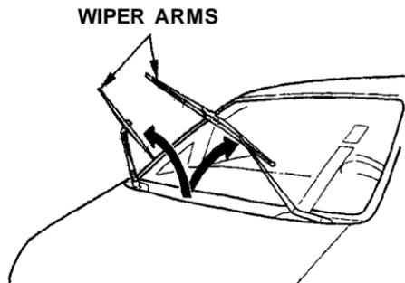
Check the condition of the windshield wiper blades at least every six months. Look for signs of cracking in the rubber, or areas that are getting hard. Replace the blades if you find these signs, or they leave streaks and unwiped areas when used.
