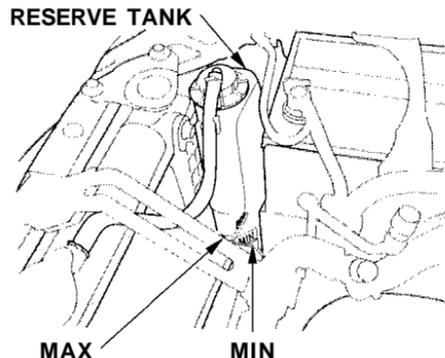
Look at the coolant level in the radiator reserve tank. Make sure it is between the MAX and MIN lines. If it is below the MIN line, see **Adding Engine Coolant** on page [152](#) for information on adding the proper coolant.
