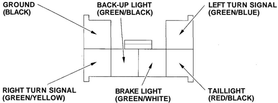
Your car has a trailer lighting connector. To use the connector, remove the left rear light cover. Refer to the drawing above for the wiring color code and purpose of each connector pin.
