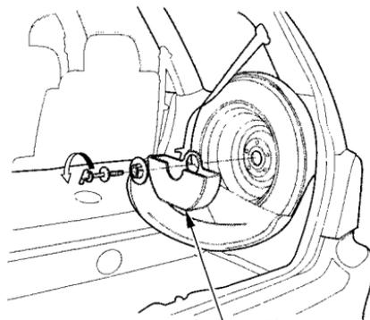
8. Unscrew the wing bolt. Remove the storage bin and spare tire.
