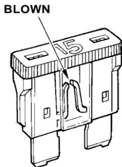
5. Look for a burned wire inside the fuse. If it is burned, replace it with one of the spare fuses of the same rating or lower.
