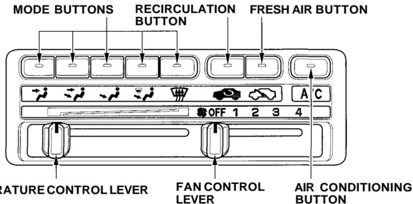
When the interior has cooled down to a more comfortable temperature, close the windows and set the controls as described for normal cooling.
