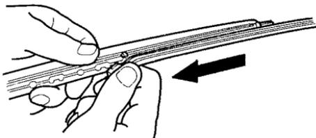
5. Slide the new blade into the holder. Make sure it is engaged in the slot along its full length.
