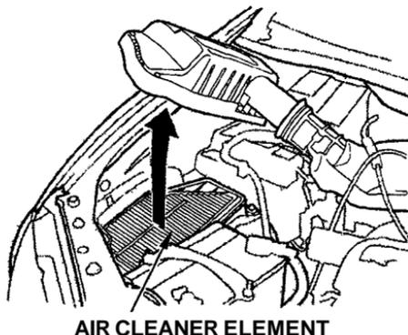
5. Place the new air cleaner element in the air cleaner housing.
