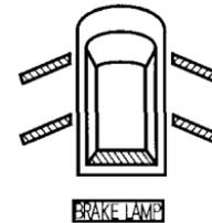
The appropriate light comes on in this display if the tailgate or any door is not closed tightly. If a brake light does not work, the **BRAKE LAMP** indicator comes on when you push the brake pedal with the ignition switch ON (II).
