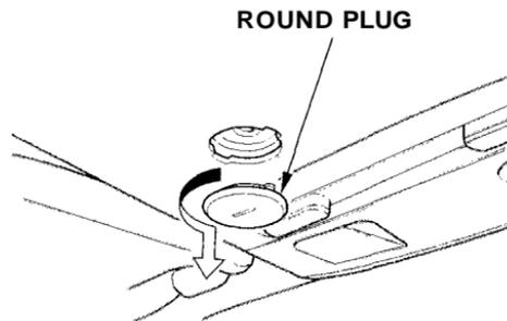
4. Use a screwdriver or coin to remove the round plug in the headliner between the sun visors.
