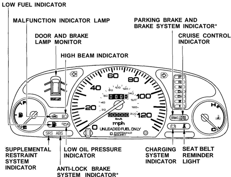
\* The U.S. instrument panel is shown. Differences for the Canadian model are noted in the text.
